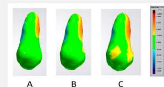
Figure 3: Colour maps showing quantitative differences between the actual and printed tooth. (A) OJ model; (B) FL model; (C) RS model
