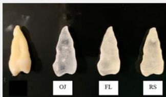
Figure 1: Depicts the extracted tooth as well as the printed OJ, FL and RS replica respectively
